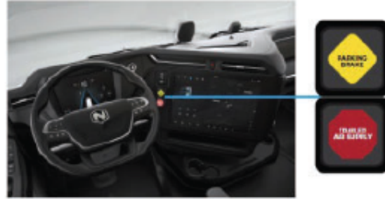
B. Activate the parking brakes by lifting up on the right side of both the yellow and red switches
