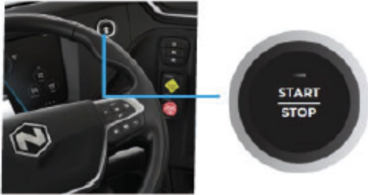
C. If the vehicle is on, and time allows, turn it off by pressing the START | STOP button
