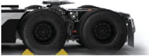
A. Chock the trailer and truck wheels
