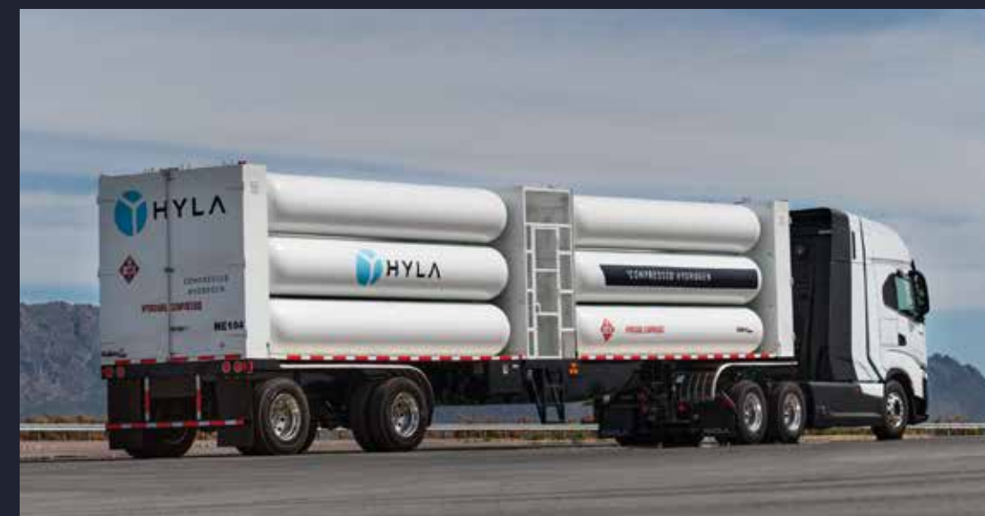
HYDROGEN TUBE STORAGE TRAILER
