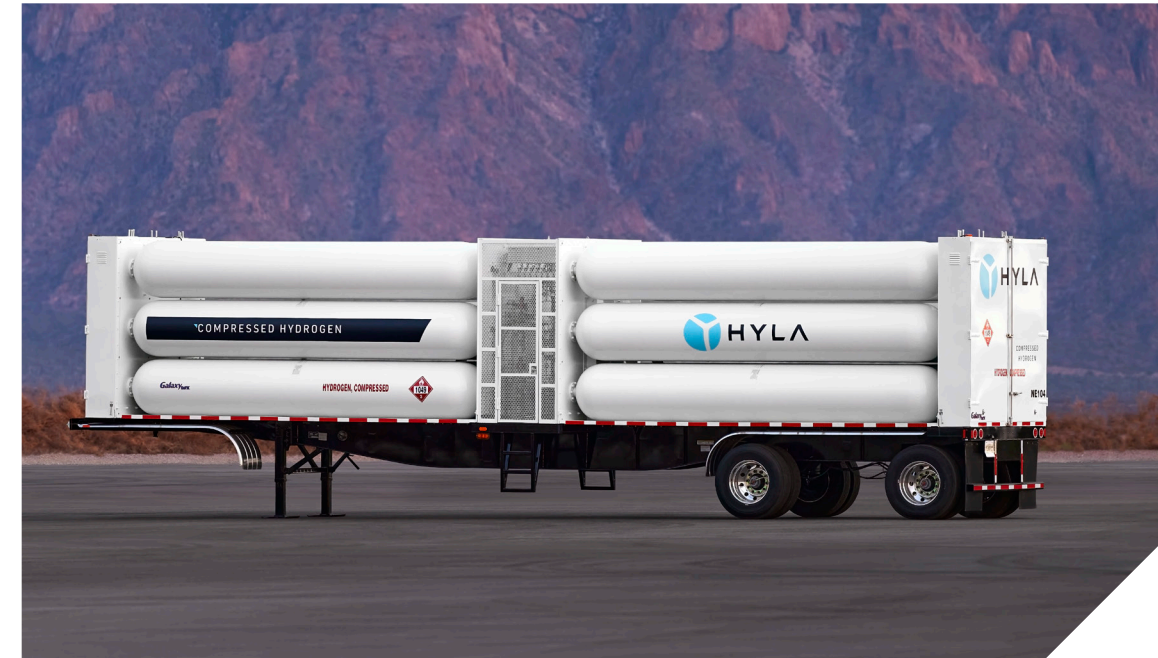
HYDROGEN TUBE STORAGE TRAILER
